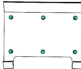
2. Make sure that you removed the transit bar from underneath the product! Without its removal, the dryer will not work correctly!
