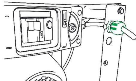
3. Pull out the waste hose entirely by pulling downwards until you see the white mark. If you do not see the white mark, the waste hose is not pulled out enough! Operating product without properly pulled out waste hose can lead to a damage to the product! Shorten the drain hose as needed.
