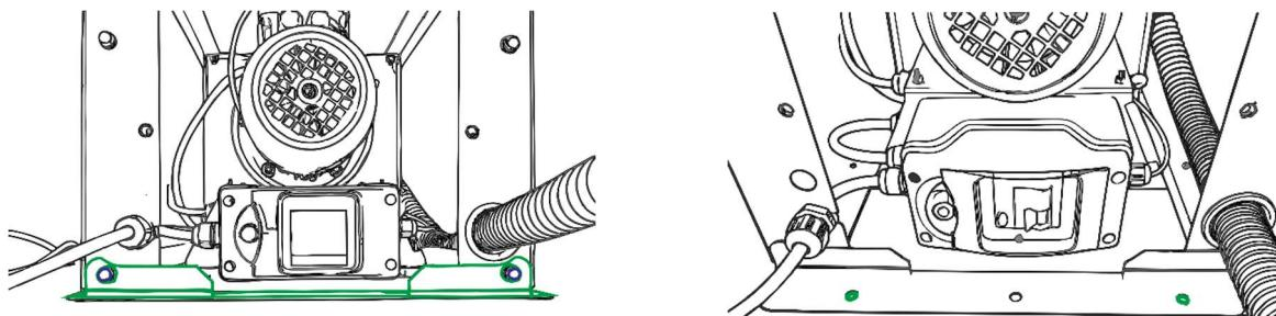
8. The RCCB is in the TRANSPORT MODE, turn it ON by flipping the switch.
