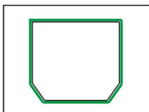
5. Apply clear sanitary sealant around the hole for inserting the swimwear spin dryer (green line).
