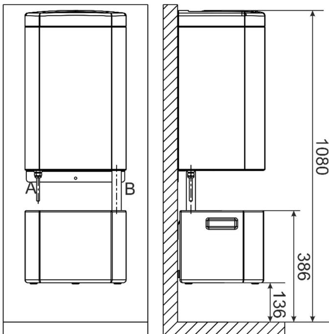
You can connect the drain hose to a water container that is installed on the wall underneath the dryer. The capacity of the water container is 18 liters of water, and it needs to be emptied manually.
