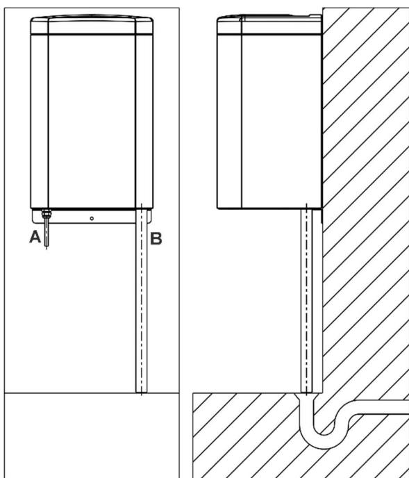
The drain hose can be connected or placed near a floor drain.
